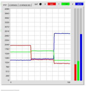
The newly added LED **SAT** indicates if one of the channels is in saturation. In this case, it lights up red.
